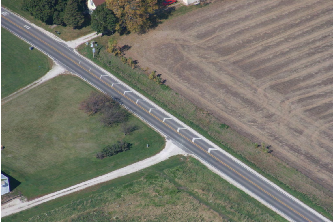
Figure 3.23. Use of converging chevrons in Roland, Iowa
